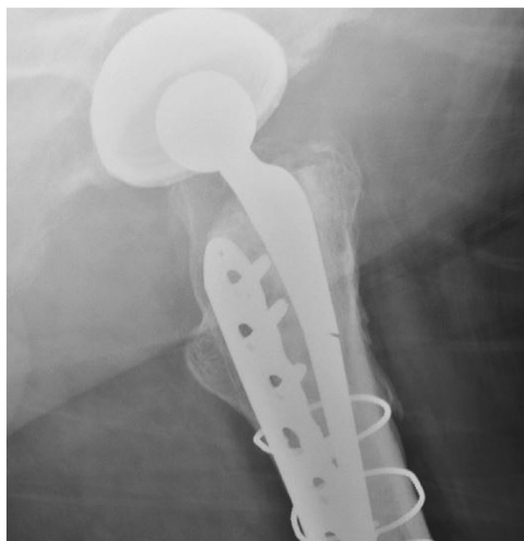
Figure 4. Lateral radiograph of the hip showing a stem fracture of a short Exeter stem.
